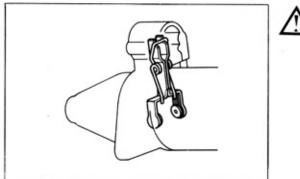
Assemble drive lever in direction as shown.
