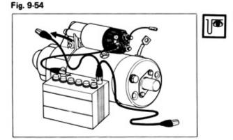
Hold-in test Next disconnect the "C" terminal. The pinion should remain in jumped-out condition.
