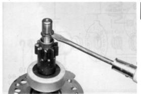
Pry the snap ring, using a screwdriver.
