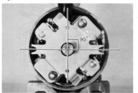
After installation, position the holder as shown.
