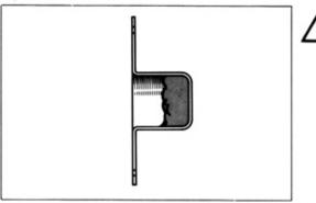
Install end frame cap not more than half full of grease.
