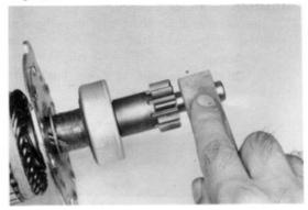
If difficult to pull out the pinion, repair the shaft with an oil stone.
